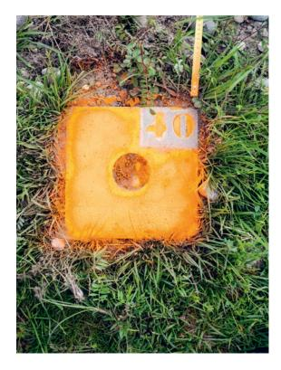
Lovász placed marker stones in the ground so that the survey locations could be found again. It is vital that the researchers always analyze exactly the same location so that the data can be compared. GPS data are too imprecise because they vary slightly from one measurement to another. The orange color makes it easier to find the stones, which have often become overgrown over the course of the year. In total, there are 80 such stones spread across the island. (left)
